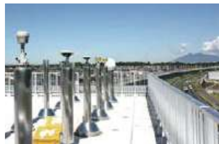
Reference baseline field for GNSS survey instruments
