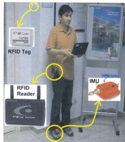
Pedestrian Indoor Navigation by aiding a Foot-mounted IMU with RFID Signal Strength Measurements Antonio R. Jimenez Ruiz, etc (IPIN2010論文集より引用)
