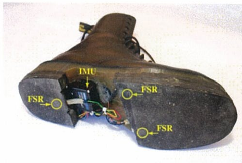
Evaluation of Zero-Velocity Detectors for Foot-Mounted Inertial Navigation Systems Isaac Skog, etc, (IPIN2010論文集より引用)
